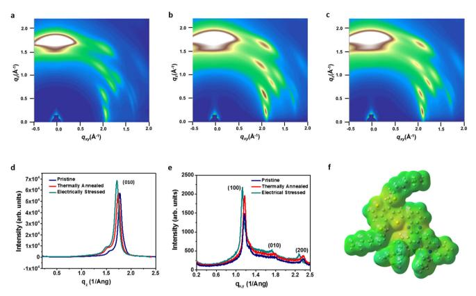
**Fig. 4 Crystallinity of the 2D conjugated polymer.** GIWAXS images of the PBDTT-BQTPA thin film **a** in its pristine state, **b** under thermal annealing and **c** upon being subjected to voltage stressing. Line cuts of the GIWAXS of the PBDTT-BQTPA thin film in **d** the out-of-plane direction and **e** the in-plane direction. **f** Electrostatic potential (ESP) surface of the repeating unit of PBDTT-BQPTA derived from molecular simulation.
